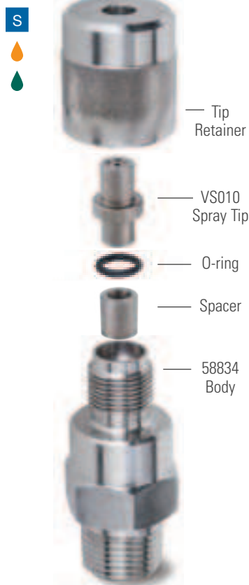
VS010 Spray Tip + 58834 Body Operating pressure up to 20,000 psi (1400 bar)
